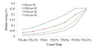
Figure 6. Analysis result of bit-line swing (with 300 mV power supply in typical process corner) at steady-state after WL enable
