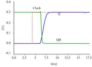
Figure 3. The simulation result of a single cell write operation.
