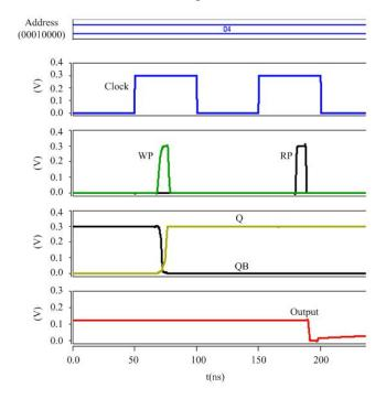
Figure 4. The simulation result of an operation cycle (one column).
