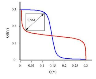
Figure 2. SNM of the proposed SRAM cell.
