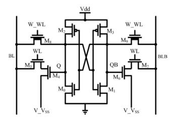
Figure 1. Proposed 10T SRAM cell.
